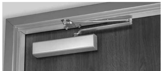
Due to the geometry of the arm it is approximately 25% less power efficient than a regular arm application. The entire closer and arm assembly are mounted below the frame stop. Top rail clearance dimensions will vary based on the type of cover used. (See pg. 15)
