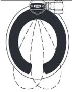
2. As the user enters the beam's effective range, 22" to 42" (559 mm to 1067 mm), the beam is reflected into the Scanner Window to activate the Output Circuit. Once activated, the Output Circuit continues in a "hold" mode for as long as the user remains within the effective range of the sensor. If the user stays longer than 65 seconds, a full flush will automatically initiate when the user leaves.
