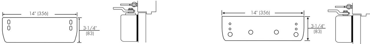
**Exposed Back - #8545A Architectural Plastic or Architectural Metal Cover Decorative Back Plate:** For use on doors with glass lights where a closer with an architectural plastic or metal cover is installed and the closer back is exposed. This plate covers the back of the installation to give a pleasing appearance from the reverse side.
