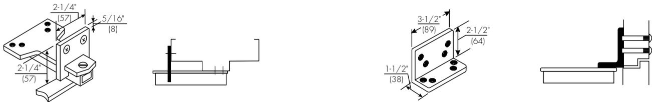
**Additional Support - #6190 Reinforcing Bracket:** Standard for use with all parallel arm *Unitrol* door controls. Provides additional support to the soffit plate on installations with door frame reveals from 1-7/8" to 4-5/8" (48 to 117mm).
