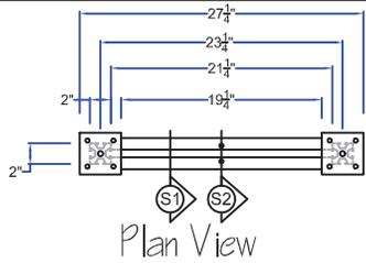
bottom track to be used as template for drilling holes for anchors in floor
