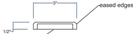
bottom track to be used as template for drilling holes for anchors in floor
